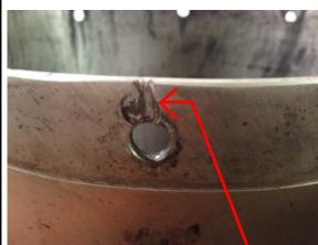
corresponding mast collar. This prevented the collar bolts from seating properly in the pre-drilled holes of the mast tube. This lack of positive engagement allowed the upper mast sections to "launch" from the lower section when pressurized, resulting in damage to the mast and the vehicles on which it fell.
